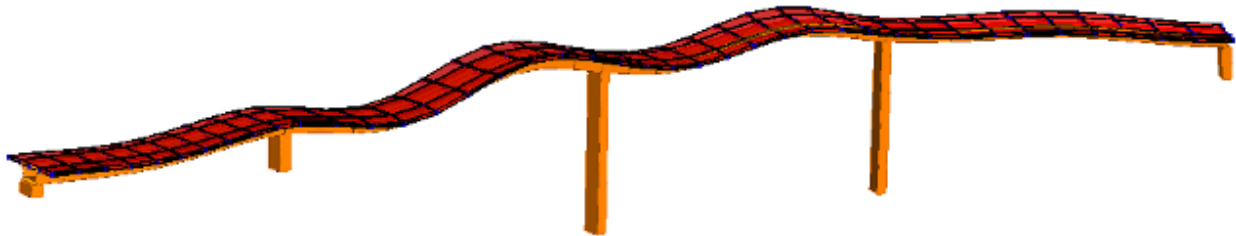
The Structure's 12th Mode ( f=4.73 Hz)
