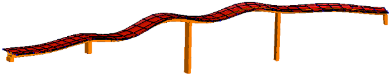
The Structure's 12th Mode ( f=4.73 Hz)
